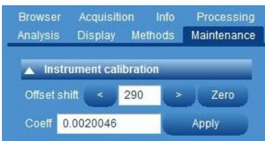
3. Keep adjusting the offset shift value until the measured peak value is within one wavenumber of the target value.
