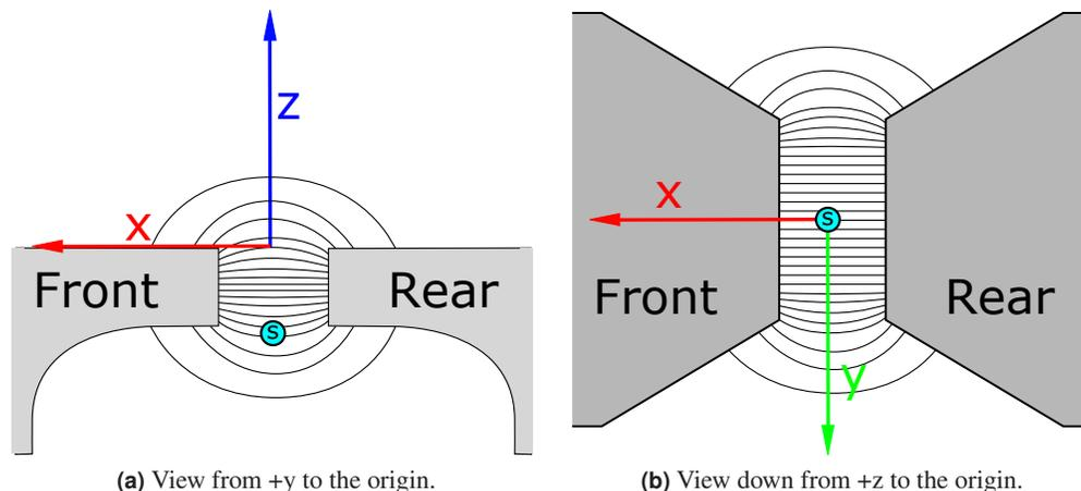
**Figure 15.6.:** Cartoons of the approximate fields between the pole faces. On the left, a side-view section, on the right a top down view. “s” denotes the position of the field sensor’s active element. The origin was chosen at the optimal point for imaging. The central position of this point will maximize the field along  $x$  and minimize the other components. The origin also best mirrors the sensor position so that the field measurement is as accurate as possible.
