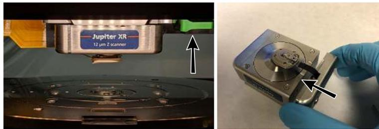
**Figure 1.6.:** The Z scanner is placed in the AFM using a dovetail geometry and secured in place by pushing the green lever up, as shown in the image. The cantilever holder is attached to the Z scanner. Each cantilever holder has a side module which contains the information relevant to each cantilever holder.
