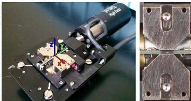
**Figure 15.5.:** Coordinate Axes defined and the field orientation. Positive sensor values are defined as B field components along the positive X-axis. To the right, a close up view of the preferred origin for imaging, which lies directly over the field sensor, highlighted as a tiny white line between the pole faces.
