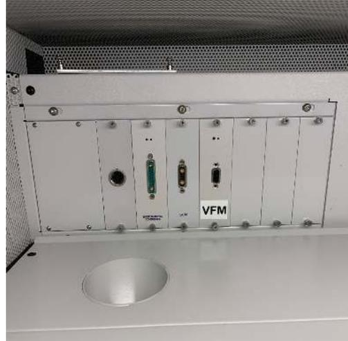
**Note** Accessories that are attached to the expansion box must be installed in order from left to right, without any unoccupied slot.
