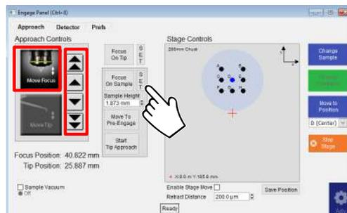
**Note** Objects up to 1.5 mm below the tip can be focused on. If the tip-sample distance is greater than 1.5 mm, the tip must be moved closer to the sample.
