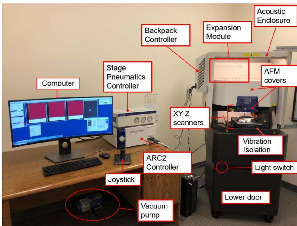
**Figure 1.1.:** The ideal set up for JupiterXR AFM.
