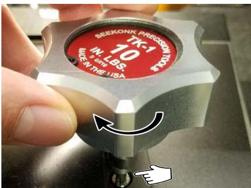
**Install the accessory chuck on the XY scanner**
