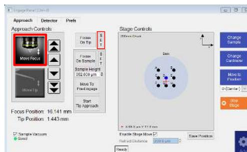
**Important** The cantilever is at an  $11^\circ$  angle, and the whole lever cannot be in focus at once. Bring the end of the cantilever closest to the tip in focus.
