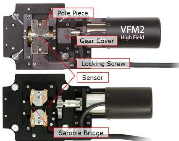
**Figure 15.11.:** Some of the basic components of the VFM defined. Also, a side-by-side comparison of the sample stages of the VFM and the VFM2-Tesla. The original VFM can be distinguished by the lacking text on the motor cover, no gear cover, and no small sensor circuit board between the pole pieces.
