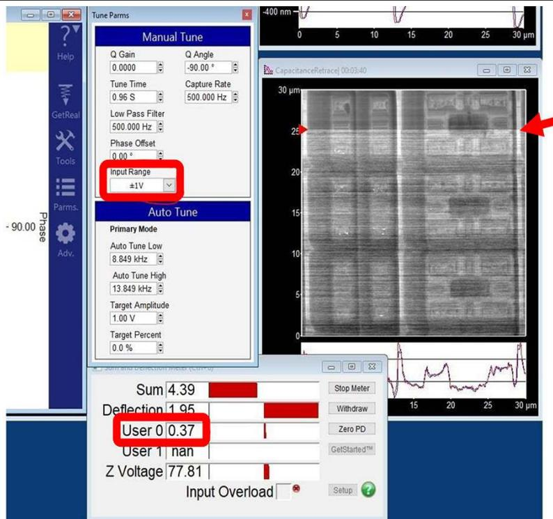
If needed, adjust the lock-in input range:
