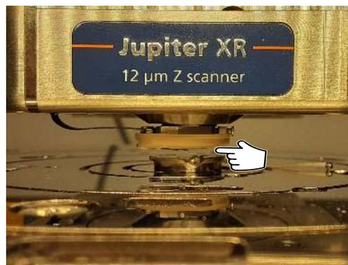
**Note** Ideally, you should have about a 1mm wide gap between the probe and sample surface.
