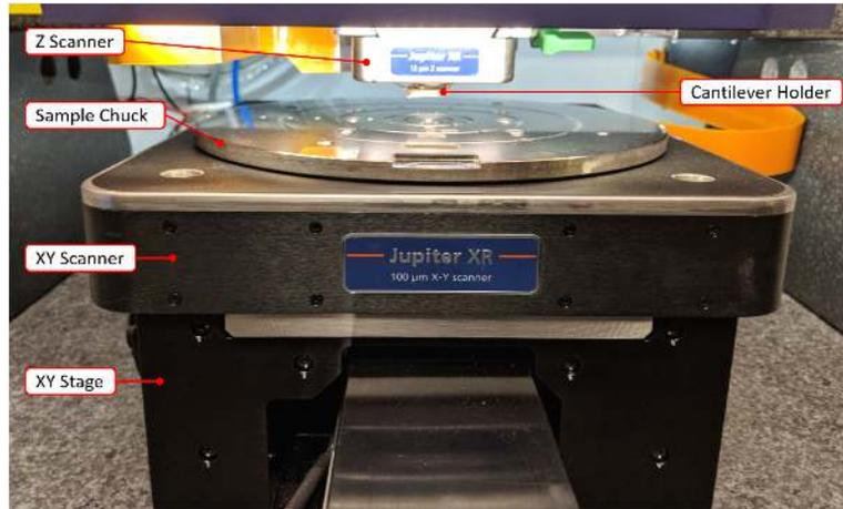
Figure 1.3.: Z scanner, XY scanner, sample chuck, and cantilever holder.
