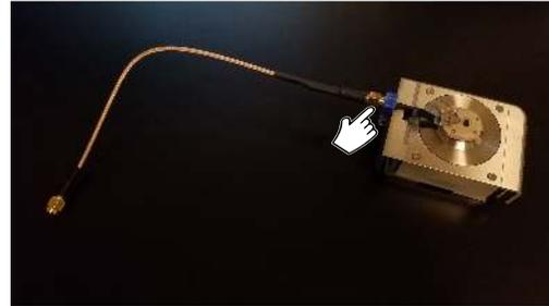
**Install the cantilever holder and SMA cable on the Z scanner**
