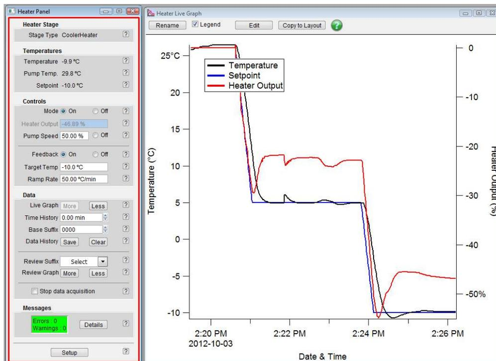
**Figure 11.2.:** Test of the cooler heater. What you might expect to see. Note that the temperature control will be less noisy if the cell is covered. You will discover this when using it inside the AFM.
