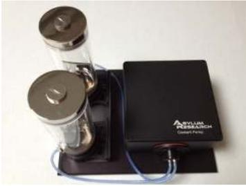
A black rectangular coolant pump assembly with two clear cylindrical reservoirs on top and a blue tube connected to the bottom. |
