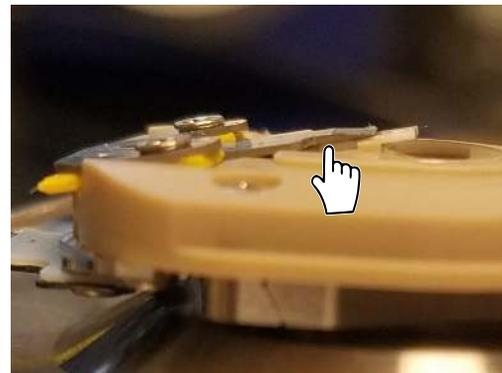
**Place the Z scanner, SCM cable, and sample**
