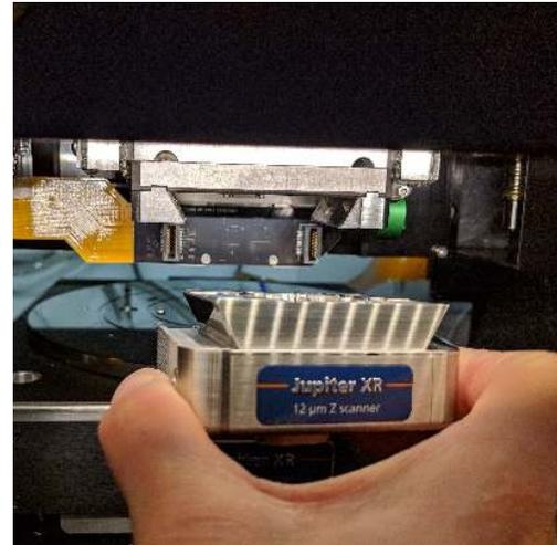
**Remove the Z scanner/ cantilever holder from the AFM:**
