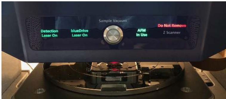
Figure 1.2.: LED indicators on the AFM cover
