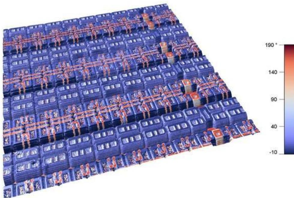
Figure 12.1.: 3D Rendition of SRAM Sample Imaged in SCM Mode.
