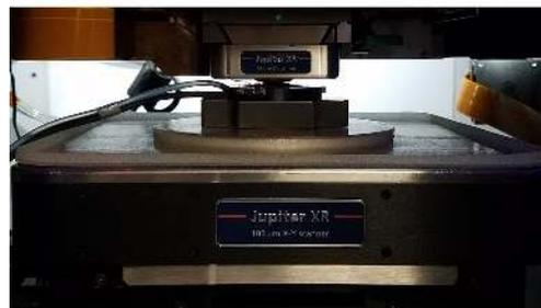
**Caution** Do NOT move the stage around with the joystick in this position or you risk damaging the Z scanner, PolyHeater stage, or accessory chuck!
