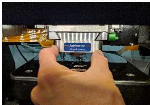
**Secure the Z scanner/ cantilever holder assembly in the AFM:**
