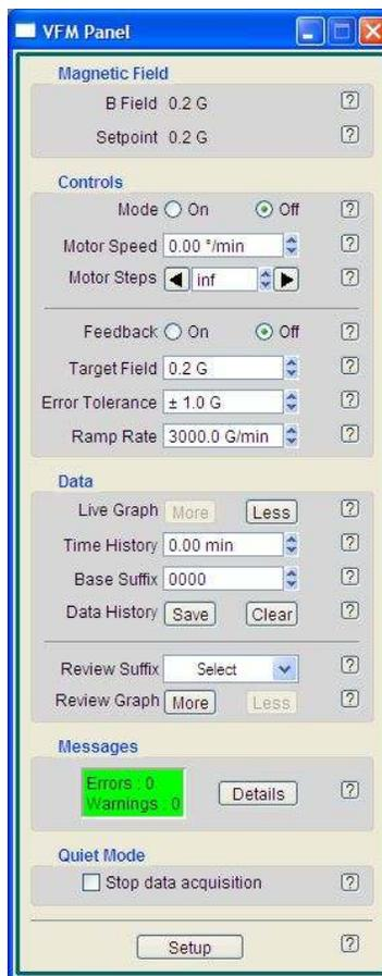
**Figure 15.4.:** The VFM panel. A complete description of each control parameter in the panel can be found by clicking on the box with the question mark next to the parameter of interest.
