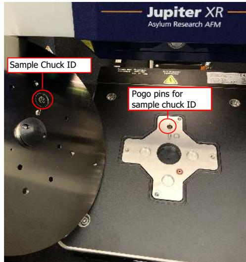
**Figure 1.5.:** Each sample chuck has an identification contact pad (ID). When the chuck is placed on the XY scanner and the pogo pins connect with the contact pad, the software recognizes the type of chuck that is placed on the scanner.
