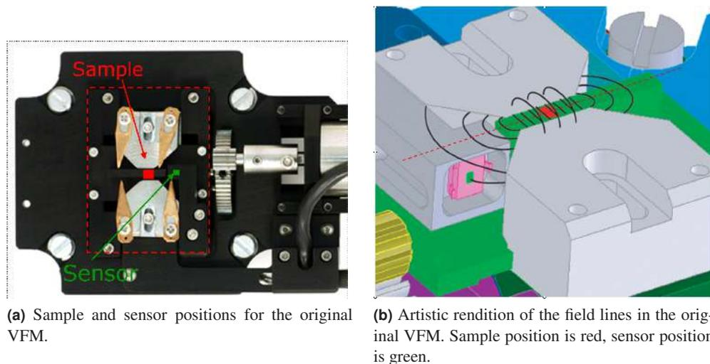
**Figure 15.12.:** The original VFM had the sensor positioned far away from the sample.
