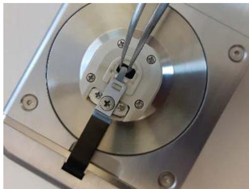
**Load a conductive probe:**
