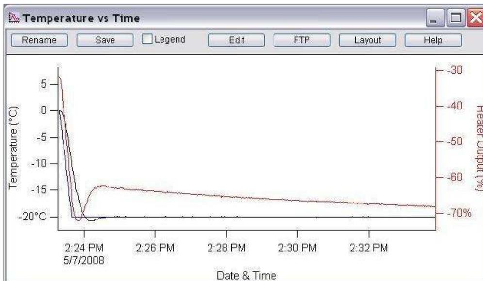
**Figure 11.4.:** The latter part of this graphs shows the heater power as the temperature ramps down to -20C. Note the steady increase in cooler power due to the body of the cooler heater warming up, and the Peltier has to work harder to maintain the temperature setpoint.
