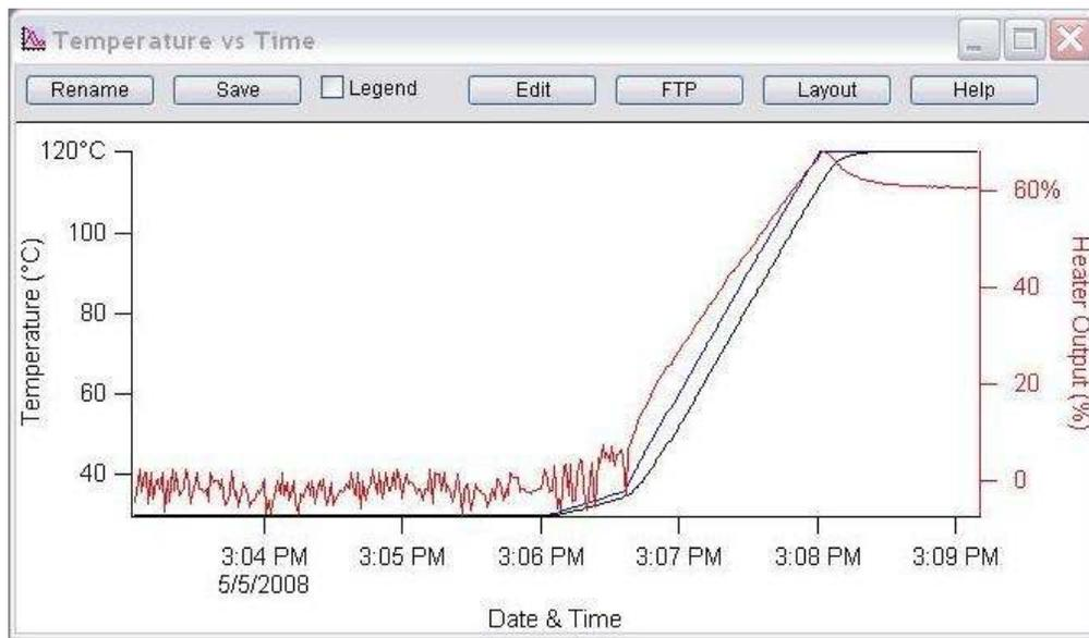
**Figure 11.3.:** The latter part of this graph shows the heater power as the temperature ramps up to 120C.
