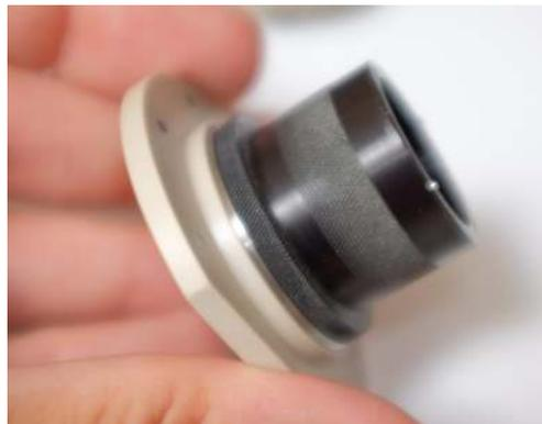
**Note** The initial threading process should be smooth. If not, you may have crossed threads - this can cause damage to the peek cell body.
