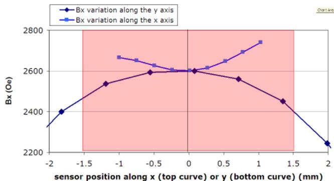
**Figure 15.9.:** Variation of the x component of the magnetic field along the x and y axes (with  $z=0$ ). Pole faces were separated by  $\sim 3$ mm. x-axis data cannot extend the full 3mm range due to the sensor plastic enclosure hitting the pole faces. The pole faces are also 3mm wide and so the red area indicates measurements taken with the sensor in the gap between the faces.
