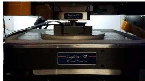
**Caution** Do NOT move the stage around with the joystick in this position, or you risk damaging the Z scanner, cooler heater stage, or accessory chuck!
