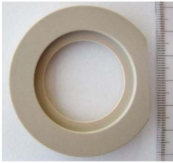
A white, circular, ring-shaped portless fluid dish shown next to a ruler for scale.     |
