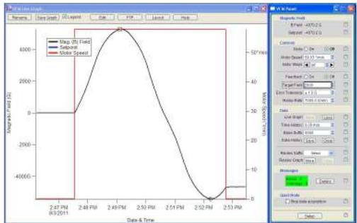
4. If the maximum field reached is more than what you need, we advise that you separate the pole pieces a little to reduce field gradients and the error in the sensor reading. Remember, if the vertical sample position is off by even 50  $\mu\text{m}$  when operating in the strongest field (smallest pole face separation), you may have absolute error in field reading by hundreds of Gauss.
