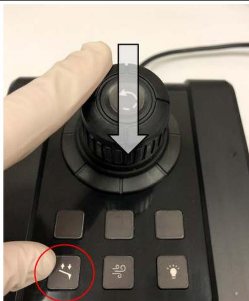
**Warning:** Nothing but your attentiveness will prevent the cantilever holder from crashing into the sample. If you crash the cantilever holder, you may cause *SEVERE* damage to your cantilever holder and scanner.
