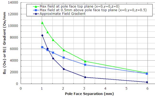
**Figure 15.8.:** Maximum field along the x-axis measured at the origin (sample in plane with pole face tops) and 0.5mm above (0.5mm thick sample resting on pole face tops). Also, the approximate field gradients at each point for  $Z=0$ .
