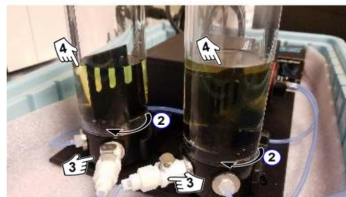
**Assemble coolant reservoir towers:**
