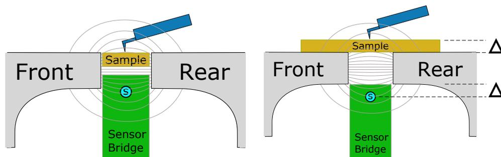
(a) Side view of a small sample between the pole faces.
