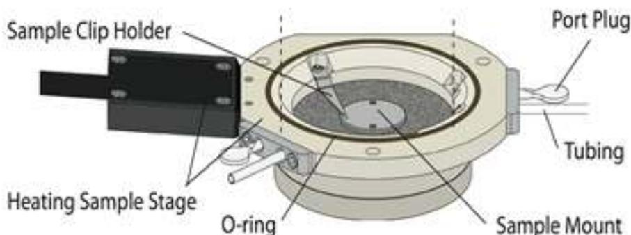
Figure 10.2.: A nice overview of the Polymer Heater and its parts.
