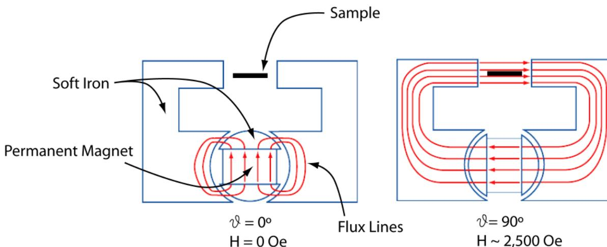
**Figure 15.1.:** How it works: A rare earth permanent magnet is at the heart of the VFM. The strength and sign of the magnetic field applied to the sample depends on the rotation angle of the magnet. When the magnet is at  $0^\circ$  or  $180^\circ$ , the magnetic flux is shunted away from the sample by the soft iron armature and pole pieces. As the magnet rotates, more and more flux is channeled instead through the sample. At  $90^\circ$  and  $270^\circ$ , the field magnitude is maximized.
