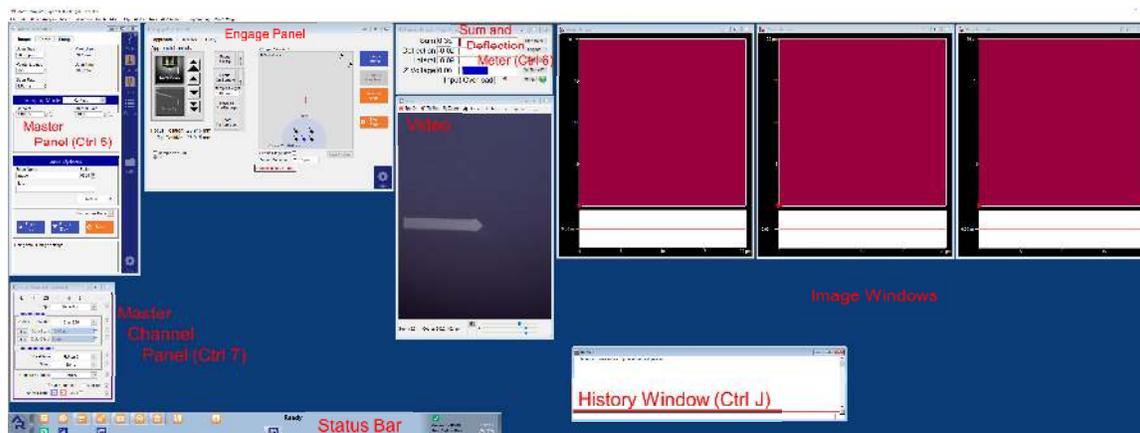
**Figure 2.1.:** Typical start up screen for the Asylum Research AFM Software after the Mode Master Panel has been closed. (A few image panels have been left off the right of the screen, which usually extends across the second monitor of your system.)
