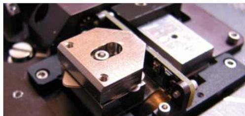
9. Repeat this process for the other pole face, making sure the two pieces are equidistant from the sensor bridge.
