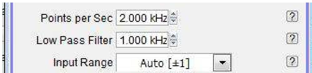
**Figure 8.7.:** [Filtering] You can set the digital filter to as low as needed. below 50Hz artifacts may appear. Be sure your filter is set to at least twice the frequency of your drive wave. note that complex wave forms (non sinusoidal) require much higher bandwidths to drive and acquire.
