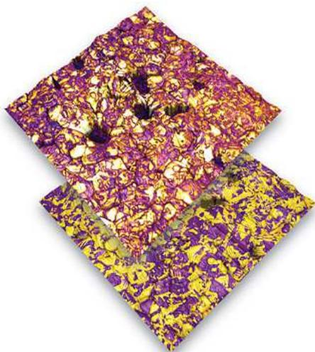
**Figure 7.1.:** PFM amplitude channel overlaid on AFM height (top) and phase image overlaid on height (bottom) of lead zirconium titanate (PZT), 20  $\mu\text{m}$  scan.
