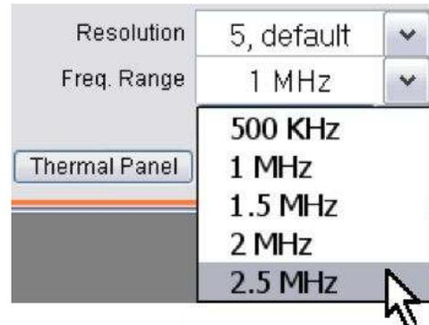
Be careful when selecting the 2.5 MHz Range on an MFP3D, as you can see all the way to Nyquist, the anti alias filters may not have removed all of the aliasing: signals between 2 and 2.5 MHz may actually be from 2.5 to 3 MHz.
