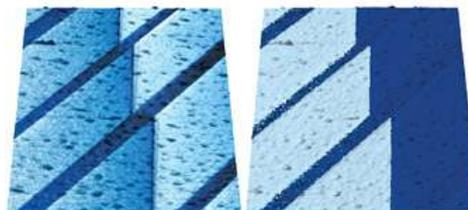
**Figure 7.2.:** PFM amplitude overlaid on AFM topography (left) and PFM phase overlaid on topography (right) on (100) oriented BaTiO<sub>3</sub> single crystal (from Castech Crystals). The amplitude and phase image show 90° and 180° domain walls in BaTiO<sub>3</sub>. 10  $\mu\text{m}$  scan courtesy of V. R. Aravind, K. Seal, S. Kalinin, ORNL, and V. Gopalan, Pennsylvania State University.
