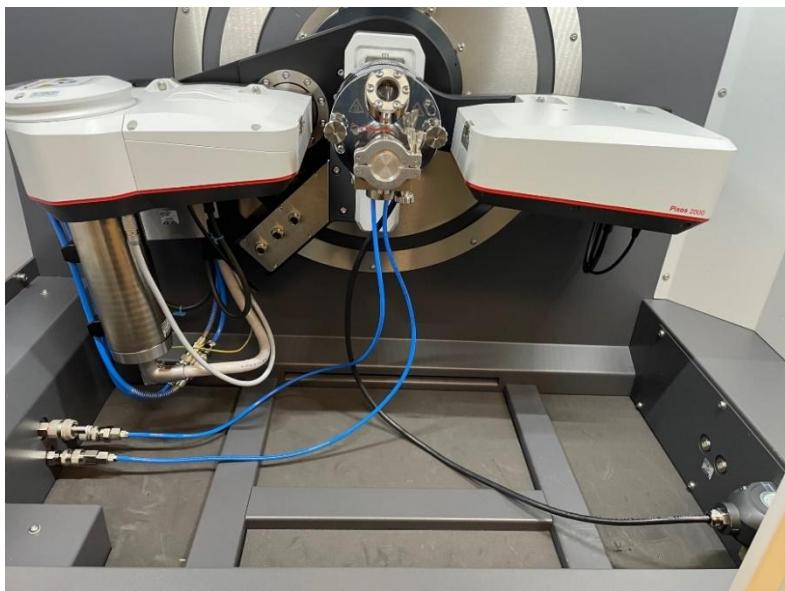
10. Load the sample into the TTK 600 stage (*see pages 27-29 in the TTK 600 guide*)
