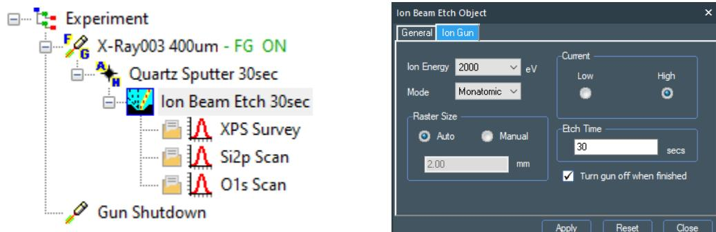
In the Ion Gun tab, select Monatomic or Cluster mode and the desired ion energy. Selecting Auto for raster size will set the etch area to be 5x the X-Ray spot size.
