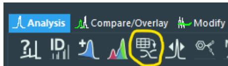
5. A dialog box is displayed that allows selection of the variable to be plotted (on the y axis) as a function of etch time (on the x-axis). A typical selection would be “Atomic %” to plot the elemental concentration as a function of etch time.
