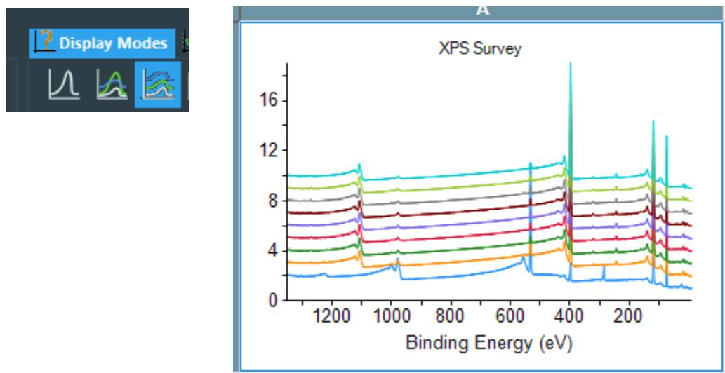
3. Create a peak table from the survey scan data or individual region scan data per the instructions found in the Data Processing and Reporting Procedure. *Note: when you perform the element ID and/or peak fitting for one of data sets in the etch series, the processing and results will propagate to all of the data sets in the etch series.*
