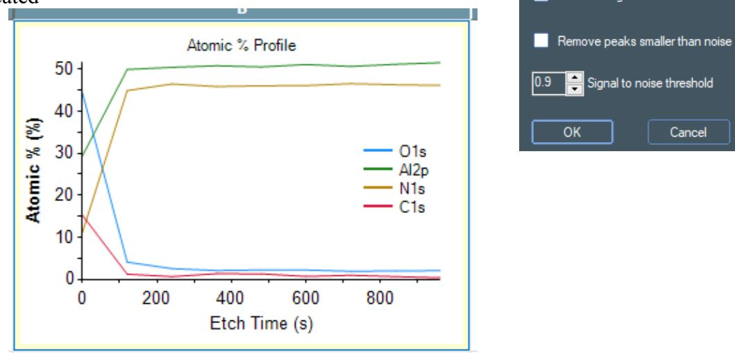
7. If the etch rate of the sample material is known or can be estimated, the etch time axis can be converted to an etch depth axis.
