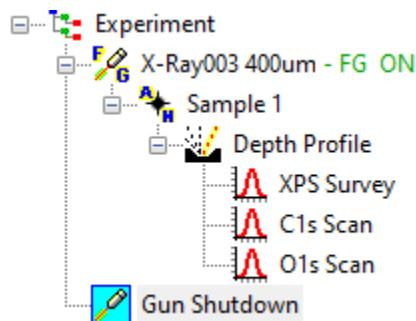
In the profile tab, select the number of total levels and the etch cycle time. Note: The number of levels is the number of measurements made, including a measurement prior to sputter etching. For example, 10 total levels would result in a measurement prior to the first etch cycle, then a measurement made after each of 9 etch cycles.
