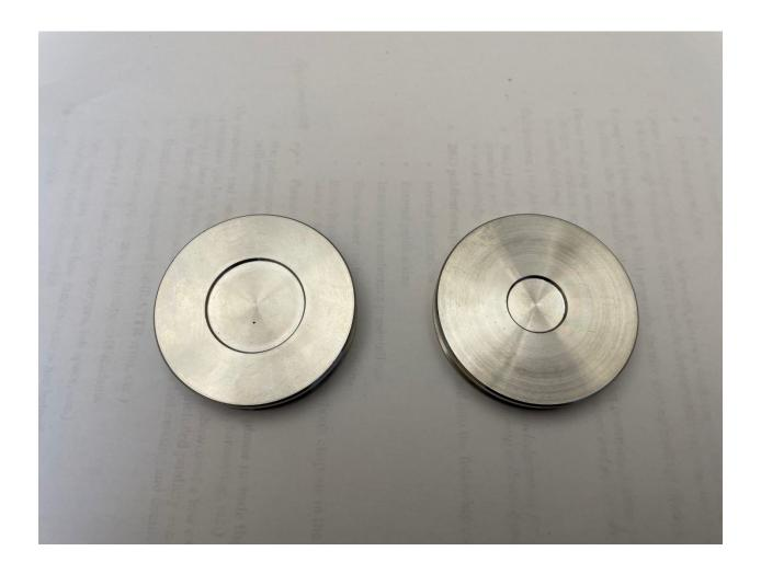
Large holder well dimensions: 25mm diameter and 1.5mm depth
