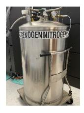
We use liquid nitrogen for many things in the laboratory. Liquid nitrogen dewars are used to fill cold traps for the Cryo-EM microscopes and some of the analytical equipment, and the boil off from a large tank is used for the supply of "house" nitrogen in the clean room.
