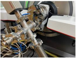
• Feed the turbo pump power cord and pressure gauge cord through XRD cabinet opening and connect vacuum hose
