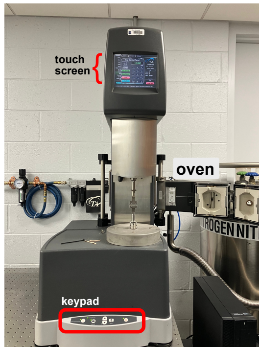
Figure 1: RSA-G2 has a touch screen displaying parameters such as Force (in [g]), Gap and Temperature . The keypad at the front of the instrument allows to move the head up and down at low and fast speeds.
