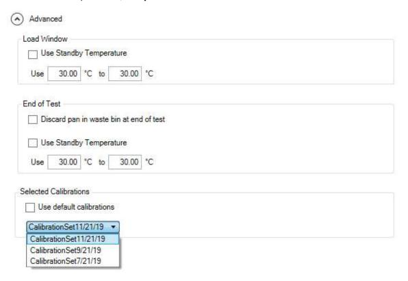
Load Window (applicable for Autosampler instruments only): This parameter is used to specify temperature range
