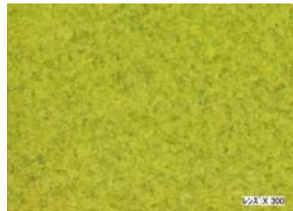
← Silicate Fluorescent Material ■ ARV-310 LED Dispersion example of orthosilicate fluorescent material (phosphor with about 15 μm particle diameter) and low-viscosity silicone resin (3 Pa s (3,000 cP)) for LED
