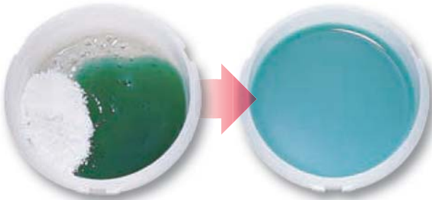
Sample-1 Epoxy Resin (base + hardener) and alumina powder
