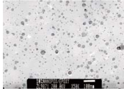
← Nano-silica ■ ARE-310 Nano-silica is uniformly dispersed throughout epoxy resin. (SEM photo by Dr. J. H. K.oo University of Texas at Austin)
