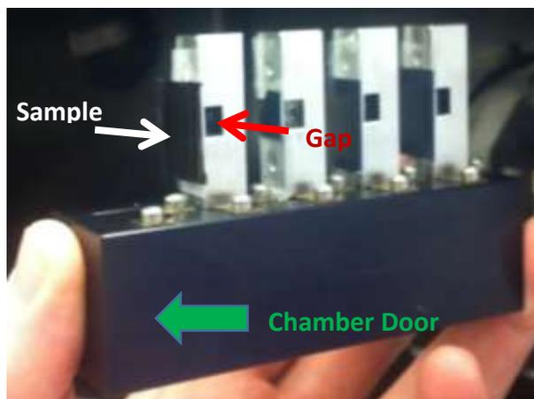
9. Mount samples on GI-SAXS stage, configuring samples as seen in above image
