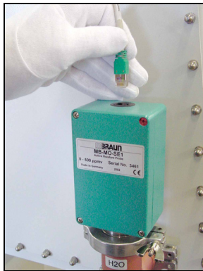
Disconnect plug connector.
