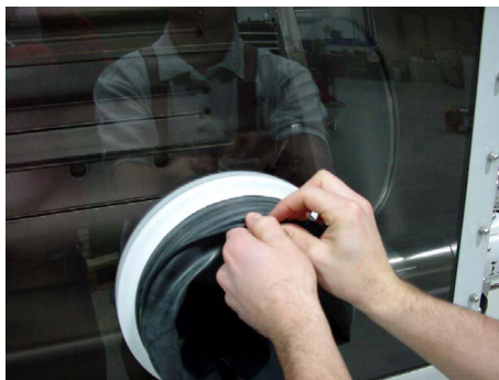
To remove the gloves remove the O-rings and removes the glove as shown
