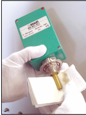
Carefully clean and dry winding.
