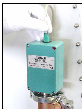
Insert plug connector.
