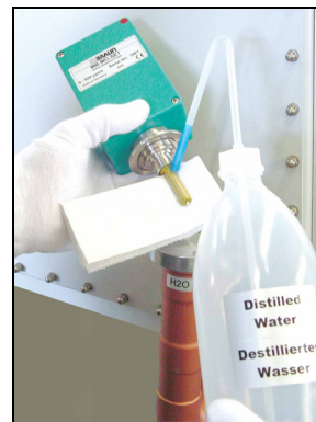
Moisten sensor with distilled water.
