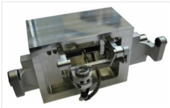
Fig. 53: Leica EM TIC 3X rotary stage for processing large sample surfaces up to 25 mm in diameter
