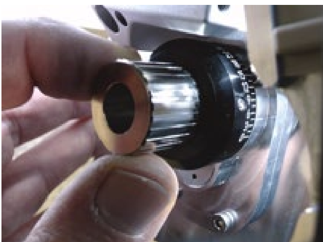
Fig. 57: Setting the milling angle (tilting angle of the sample)
