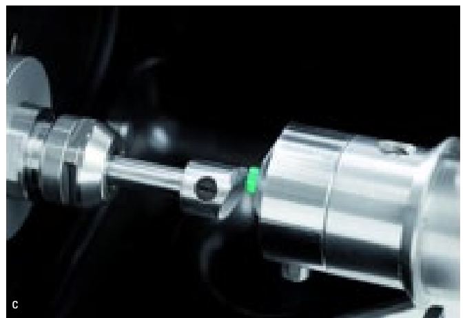
Fig. 80: Leica EM TXP with tools for polishing (a), sawing (b) and milling (c)
